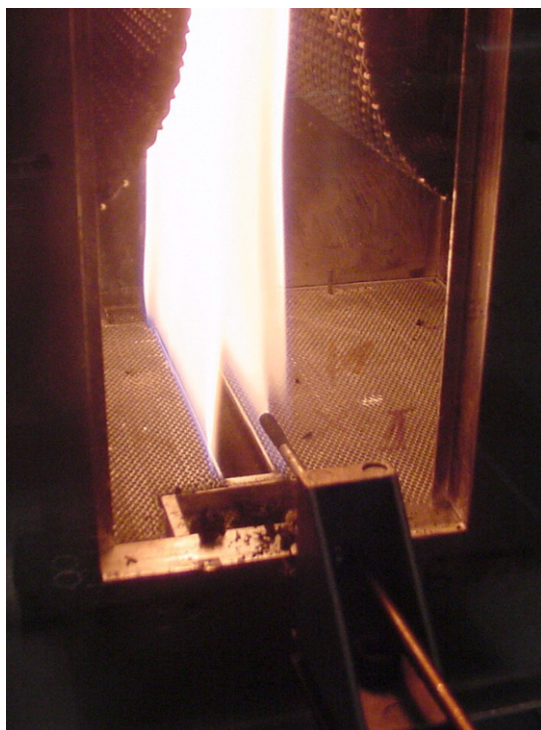
Fig. 2. Photograph of stainless steel sample probe, extracting soot from the steady ethylene slot flame.
